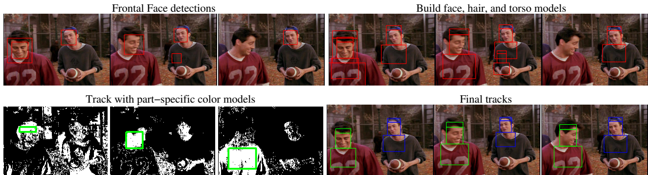
Figure 4. Low-level tracking. We first run a frontal-face detector on all frames in the video ( upper left ). For each detection, we build a color histogram model for the face, hair, and torso ( upper right ). We want to find good detections with many similar body models in neighboring frames - we do this by clustering the body models within a shot, and throwing away small clusters. We then track through frames neighboring the good clusters to find additional non-frontal poses. We track using part-specific color models built from the clusters. In the bottom left , we show thresholded likelihood ratio maps for the hair, face, and torso color models (run on the third frame in the sequence). We finally track by enforcing a rigid spatial alignment of the hair, face and torso parts ( bottom right ).
