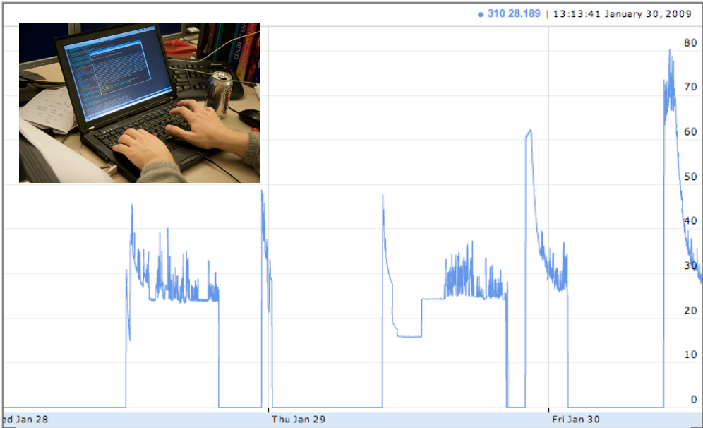
Figure 4.8: ACme reveals interesting characteristics of devices such as a laptop. We can observe the power states, charging curve, and CPU usage.
