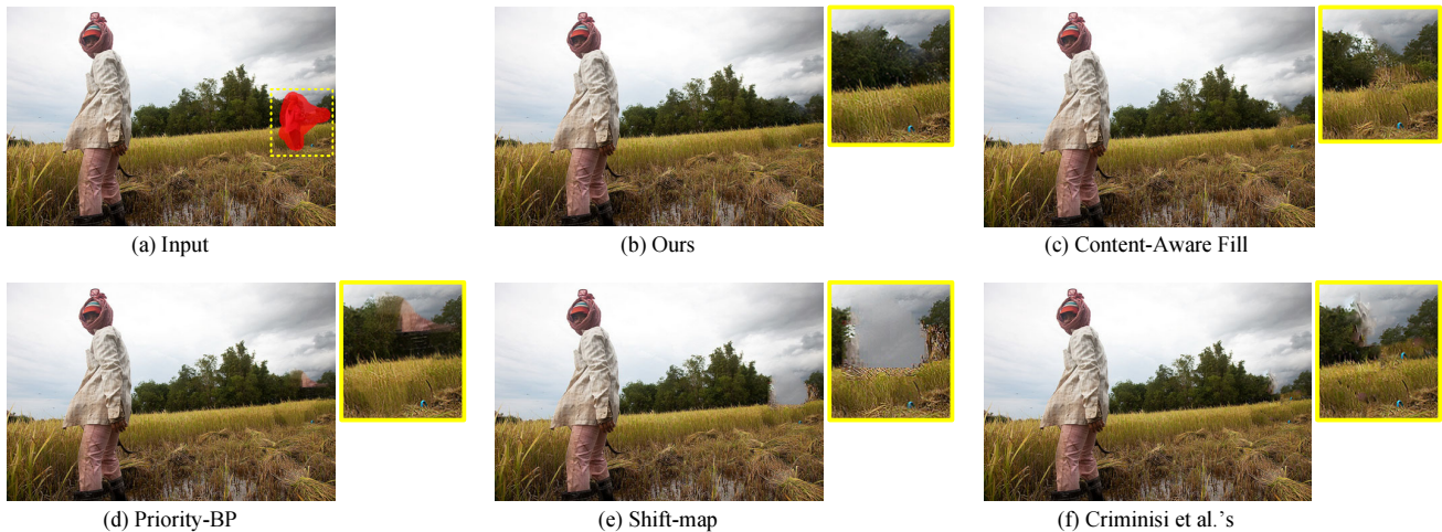
Fig. 16. Comparisons with state-of-the-art methods. (a) Input ( 640 \times 430 ). (b) Ours (graph-based, 0.18s). (c) Content-Aware Fill (0.3s). (d) Priority-BP [15] (117s). (e) Shift-map [17] (13s). (f) Criminisi et al. ’s [7] (6.9s).
