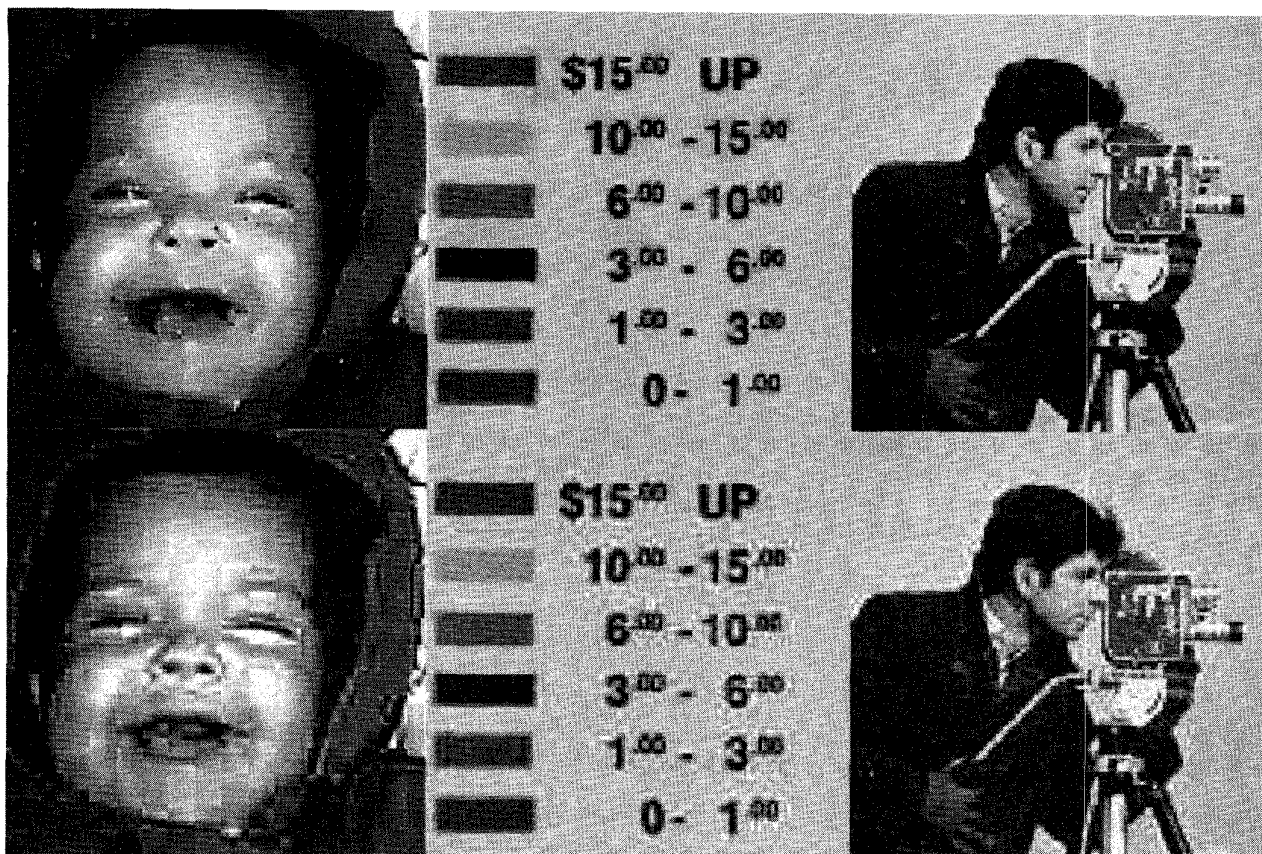
Figure 5: Zoom of reconstructed images. Top: NLP-JPEG, bottom: DCT-JPEG. Image "baby": NLP (30.04dB @ 0.45bpp) DCT (29.22dB @ 0.45bpp). Image "graphics": NLP (35.35dB @ 0.44bpp) DCT (32.70dB @ 0.44bpp). Image "cameraman": NLP (32.48dB @ 0.907bpp) DCT (30.26dB @ 0.914bpp).
